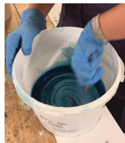
**Step three** - Make up the resin mixture. This is 50% of each part; A and B. In this case, part A has a yellow pigment, but you can customise your colour at this stage, or add other details.
