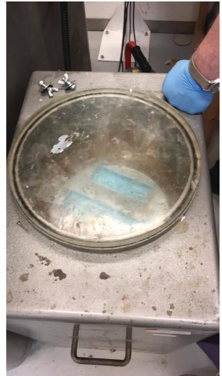
**Step four** - Pour the mixture into the mould. We used an example of a mould that had been made earlier of a shark tooth fossil.
