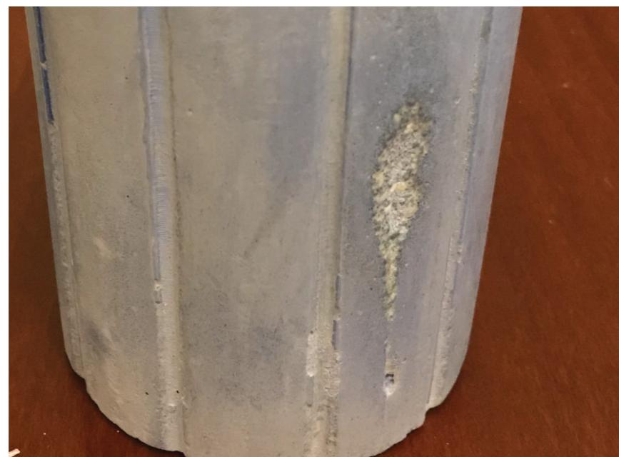
This can be resolved using tape and elastic bands to hold the mould in its shape as the concrete is placed into the mould.
