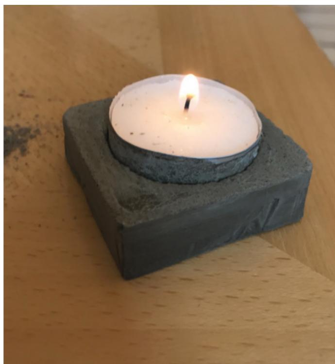
As you can see in the specimen (above on the left), there is a glossy surface finish on one of the sides. This is where there was tape on the inside of the mould. There are also air bubbles throughout the concrete. I think this is due to the inaccuracies of the mould, so I will be interested to see what happens when I have a higher standard of mould.
