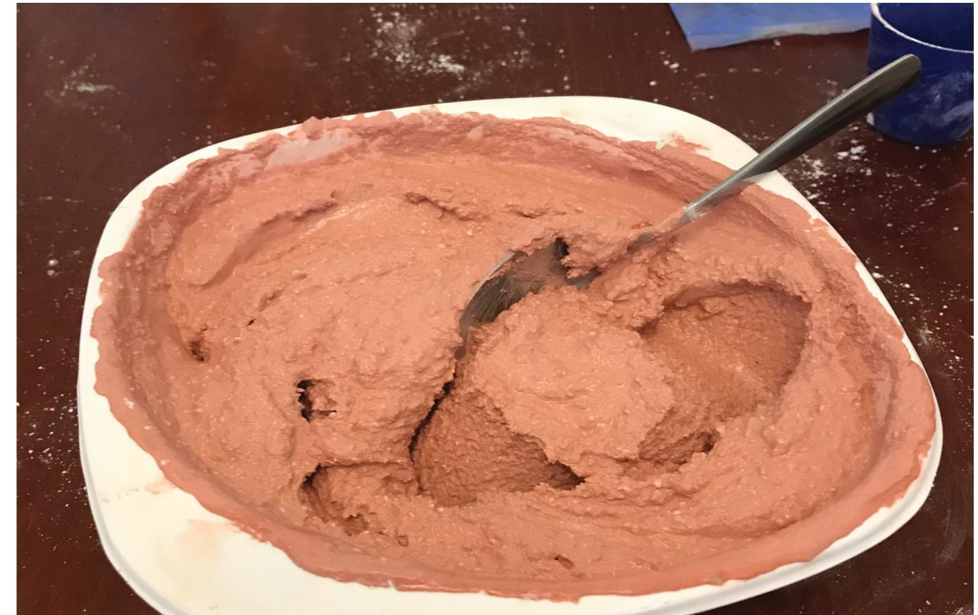
I bought some J24 fast setting silicon to make moulds of my 3D printed parts. I made two complete sets of moulds. This has been limited to two due to the cost of the silicon.
