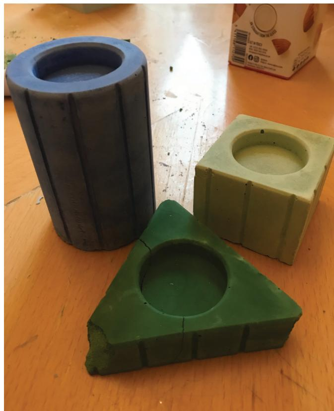
This next set has been an improvement. I used the same technique, other than mixing the pigment in water rather than straight into the powder.
