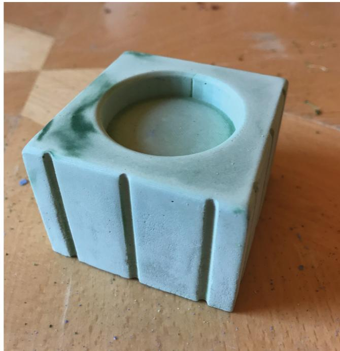
There is a slight discolouring in this holder, caused by the pigment not being evenly distributed throughout the material as it is placed in the mould.
