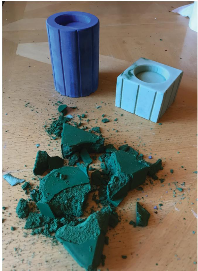
The first set to come out of the moulds was ok, however it was not the standard I was expecting, and the dark green colour concrete failed to cure and gain strength.
