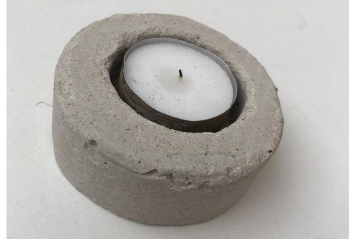
I needed to experiment further with the process that I imagine using for my candle holders later in the project, at this stage in the process. I borrowed an unused silicon mould from the workshop that was a somewhat similar shape to my initial prototypes and made up some concrete for it. The specimen on the right was made with a mixture of the two types of concrete; grey and white.
