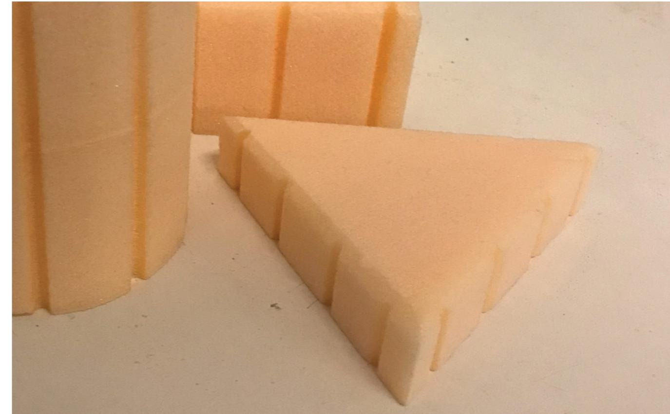
3D prints have a very obvious aesthetic. They have small ridges from each layer of the print. These would be reflected in the mould, so I attempted to finish the part to an acceptable standard. The ribs on the design were too close together and made it nearly impossible to sand away the 3D print ridges.
