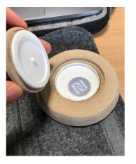
This development came from a series of issues that came about when prototyping this mechanism. The wide thread is awkward to manufacture from wood, so it made sense to introduce the plastic inserts. Plastic is easily shaped, cheap, and faster to prototype. This would also keep down the complexity of the wooden parts, simplifying the manufacturing process.
