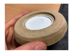
I made the prototype by cutting 3 circular layers, each with a hole in the centre. I glued each layer together and then sanded to create the chamfered edge. This took me a couple of hours to produce and due to the thickness of some of the layers this was very difficult. Even with the use of a laser cutter, this process would be done predominantly by hand. A more efficient way of forming these wooden parts is through CNC milling.
